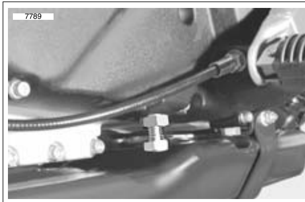
Figure 1-22. Chain Limiting Screw-without Spacer
