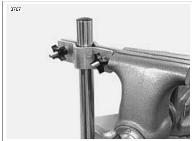
Figure 1-25. Clamping the Fork
