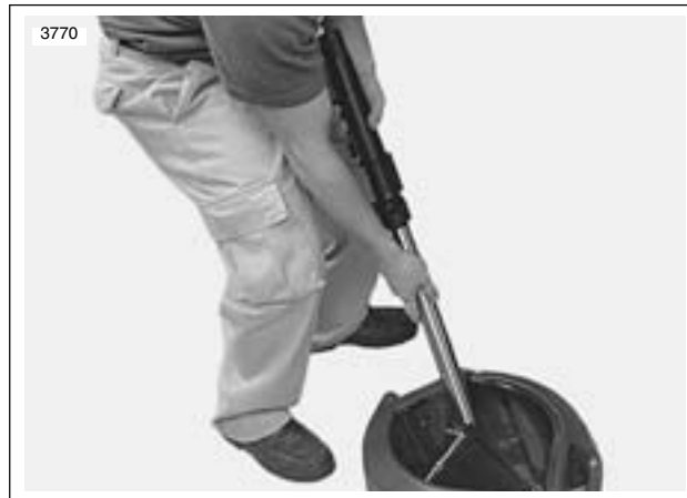
Figure 1-29. Pumping Fork Oil
