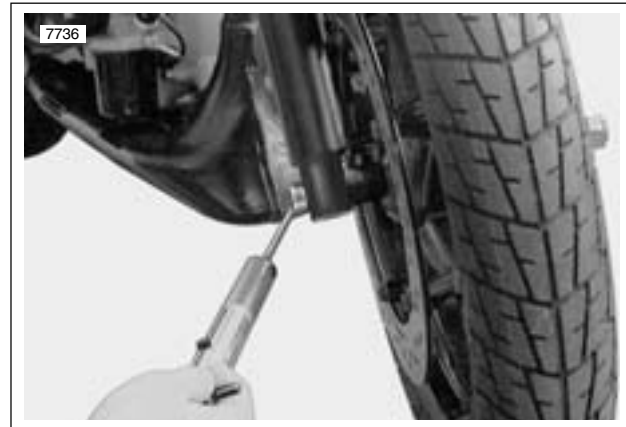
Figure 1-32. Steering Head Bearing Check
