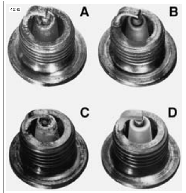
Figure 1-34. Typical Spark Plug Deposits
