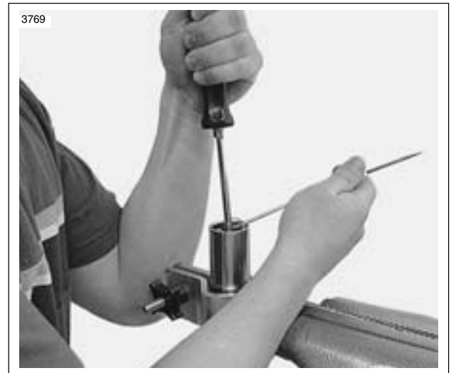
Figure 1-30. Compressing Spring Seat
