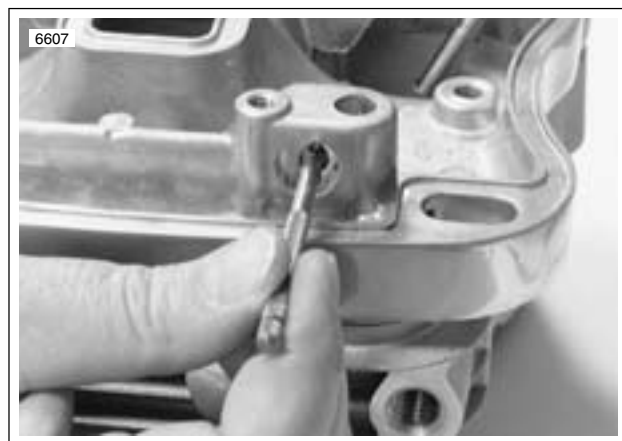
Figure 3-50. Measuring Rocker Arm Shaft Bore Diameter in Lower Rocker Cover
