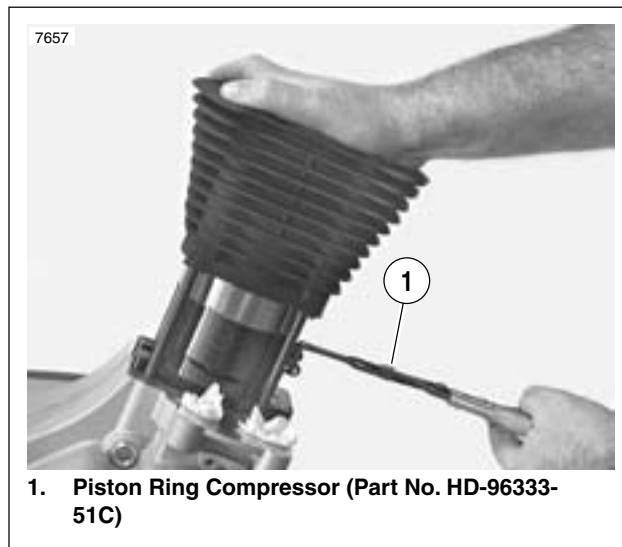
Figure 3-82. Compressing Piston Rings
