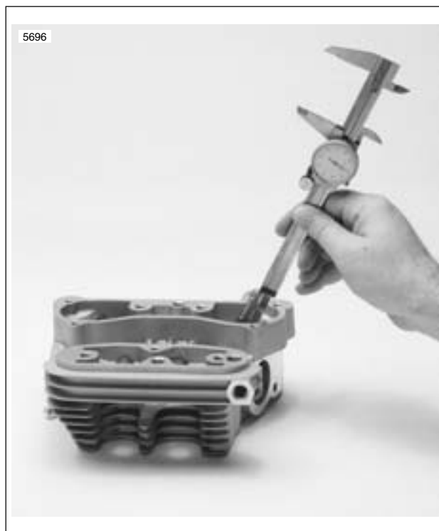
Figure 3-59. Measuring Valve Stem Protrusion
