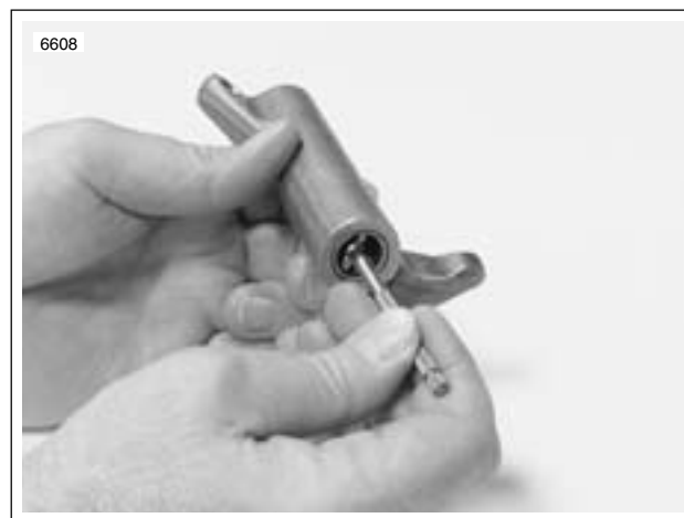
Figure 3-51. Measuring Rocker Arm Bushing Inner Diameter
