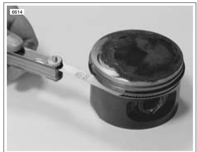
Figure 3-75. Measuring Ring Clearance in Groove
