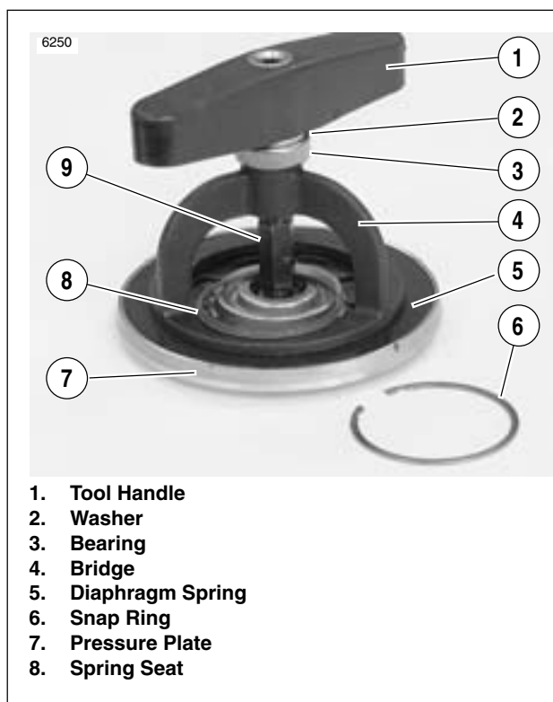
Figure 6-21. Pressure Plate Assembly
