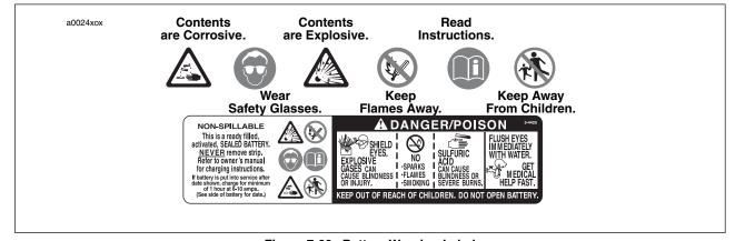
Figure 7-60. Battery Warning Label
