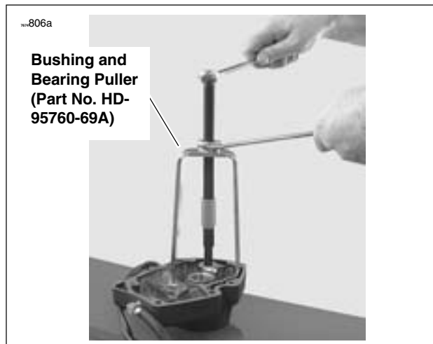
Figure 3-102. Removing Bushing
