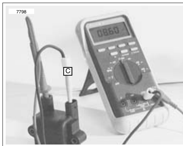
Figure 7-26. Ignition Coil Secondary Resistance Test
